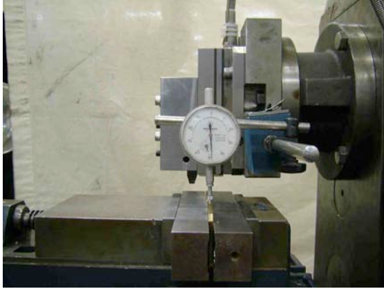
Fig. 4-3-6 Measurement of depth of cut
