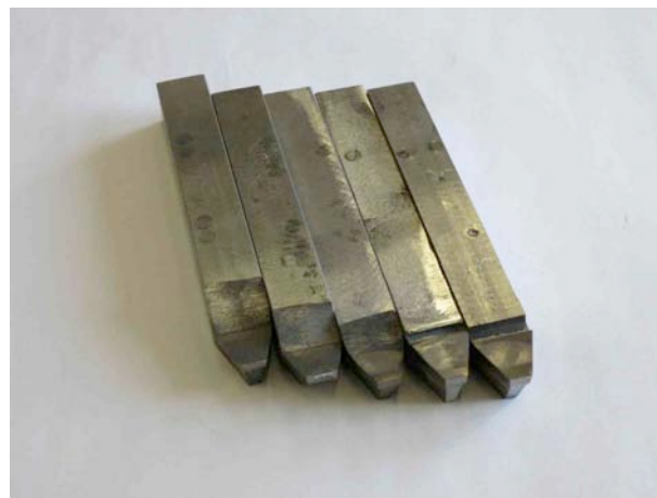
Fig. 4-3-4 Tools for orthogonal cutting
