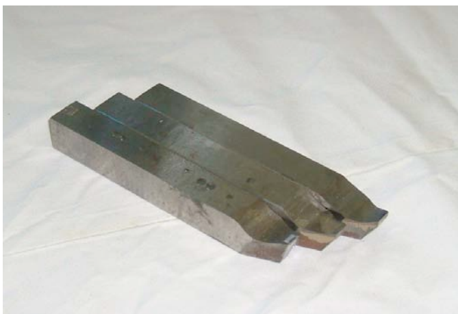
Fig. 2-3-4 Tools for orthogonal cutting
