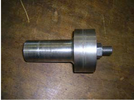
Fig. 2-3-3 Mandrel (workpiece holder) and disk-type workpiece
