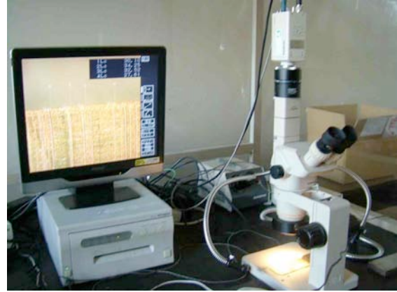
Fig. 4-3-7 Measurement of surface plastic flow
